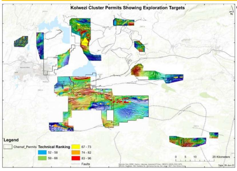
A total of 14,555 KM Airborne Geophysical survey was completed at Kolwezi Cluster permits and exploration targets identified and prioritized.
